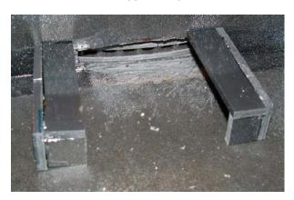
Step 7: <u>Bearing Installation:</u> There are four plastic units with roller bearings. These are to be mounted at quarter points to the underside of the turret. Locate the first bearing unit directly in line with the main gun, and the other three bearings at ninety degrees around the turret ring. It may be necessary to trim the plastic frame the roller bearing so that the plastic will not interfere with the upper hull.
