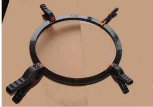
After the ring assembly has dried, remove the clamps and sand smooth the inner surface of the rings. Also sand and bevel the four edges of the ring assembly. The ring assembly will rotate with the turret, and smooth surfaces will provide much improved operation of the system.
