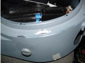
**Step 8:** Ring Assembly: There are three large ABS rings, two are smooth and one with teeth. The three rings are to be glued together, with the tooth ring in the center.
